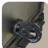
CLOSEUP OF PINTLE
