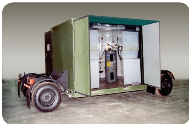
Self-contained ISU® 90 Laundry Unit shown with optional High Speed Mobility Wheel Set (P/N 60340-002)
