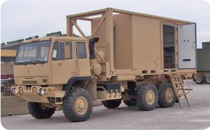
Rock Island Arsenal, Joint Manufacturing and Technology Center Petroleum Quality Analysis System Enhanced (PQAS-E) Configuration Shelter
