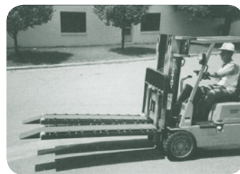
Attaches to forklift and is used to pick up pallets directly from ground. Note the beveled nose plate.
