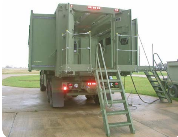
Rear view of M1087 Expandable Van Shelter shown mounted onto a FMTV 5-ton truck (stairway and platform not supplied)
