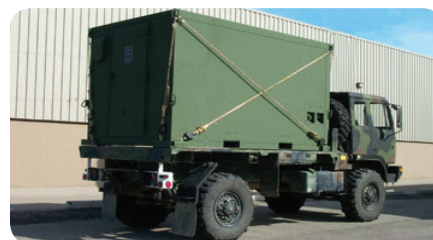
Rear view of MSC-LMTV shown with tie-down kit (PN 86060-028), designed by Peck & Hale
