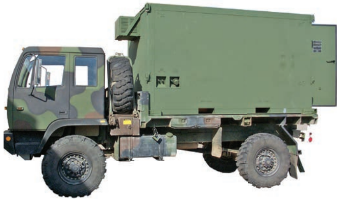
Mobility Shop Container for the LMTV is shown loaded on a standard LMTV truck
