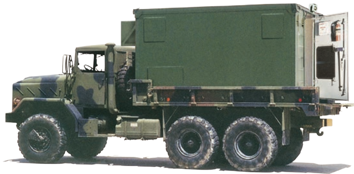
S-280 C/G Shelter shown loaded onto a 5-ton tactical truck
