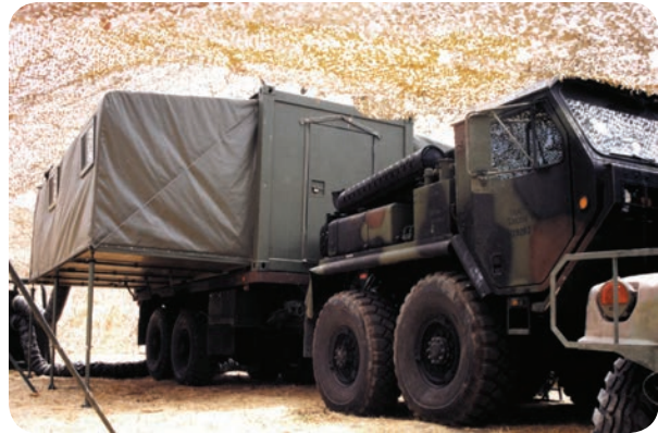
USMC deployment of rigid and rugged MECC shelter under camo netting
