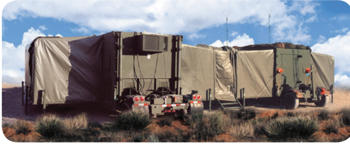
Two ELAMS TOCs deployed and complexed together
