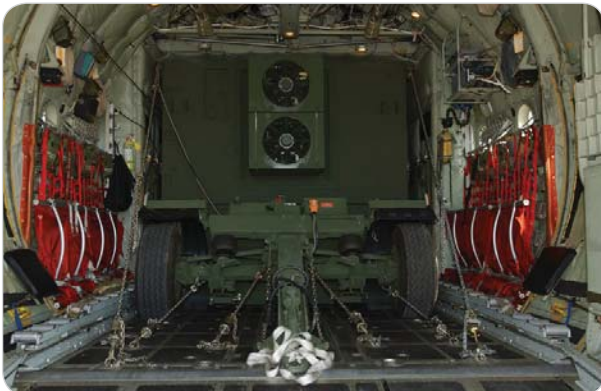
ELAMS on an optional wheel set locked in for transport in a C-130.
