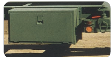
Rugged accessory/tool box mounted to frame.
