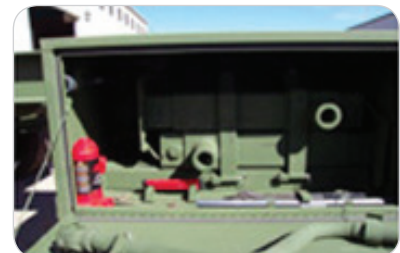
Rugged accessory/tool box mounted to frame.
