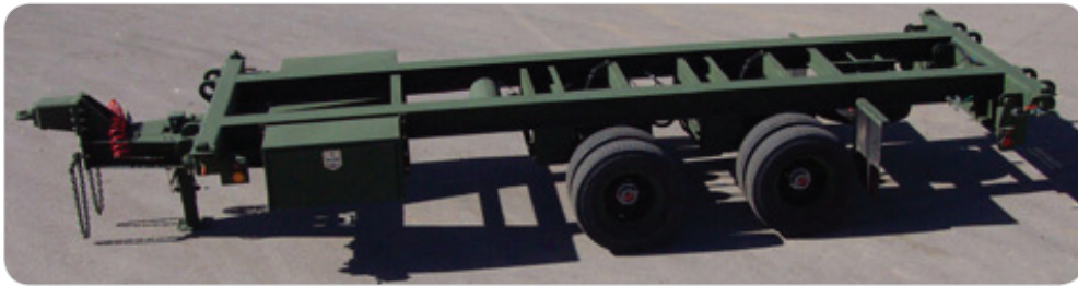
ISO Mobility Trailer - 28,000 Pound Payload Capacity.
