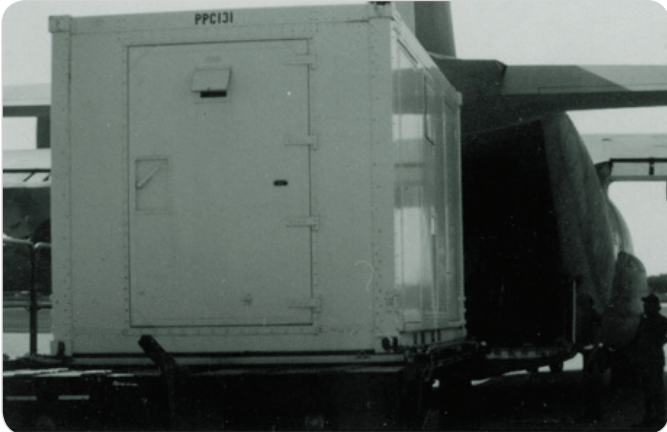
DOD Avionic Shelter attached to ISO Cargo Pallet loading into C-130 aircraft.
