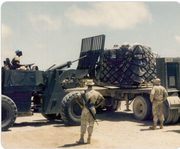
HCU-6E 463L cargo pallet with cargo restraint nets being unloaded from a truck.
