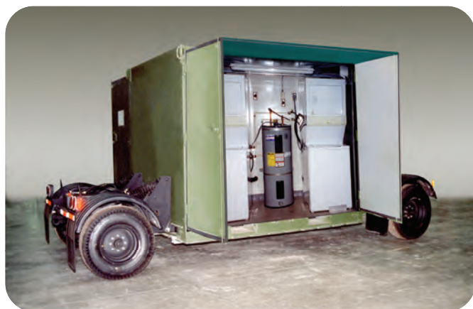
Self-contained ISU® 90 Laundry Unit shown with optional High Speed Mobility Wheel Set (P/N 60340-002)
