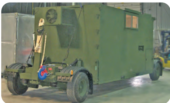
LAMS with High Speed Mobility Wheel Set, ECU, and Generator
