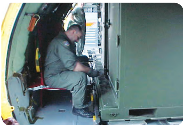
ISU 70KCA with 8" aisleway making room for seats
