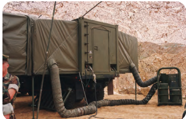
ECU with input and output hoses
