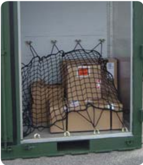
ISU Floor Cargo Restraint Net using 6/E cargo rings to anchor net.
