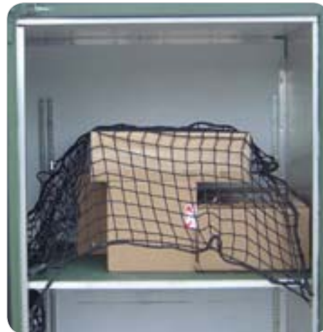
ISU Shelf Cargo Restraint Net using shelf brackets to anchor net.
