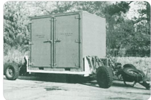
ISU-90 in position for towing using M720/832 Mobilizer Adapter and Low Speed Mobility Wheel Set.
