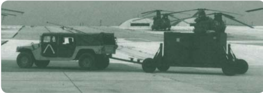
Mobility Wheel Set loaded with ISU-60.5 being towed by HMMWV.
