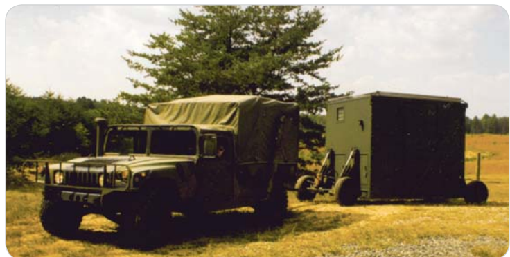
Low Speed Mobility Wheel Set used at Quantico to move ISU-90 Containers.
