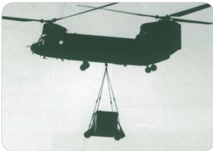
Mobility Wheel Set is helicopter slingable and truck transportable.
