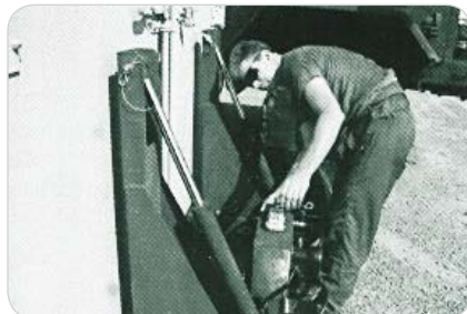
ISU Mobilizer Wheels Sets pumps use standard, military 24 volts system for operations.
