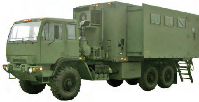
M1087 Expandable Van Shelter shown mounted onto a FMTV 5-ton truck
