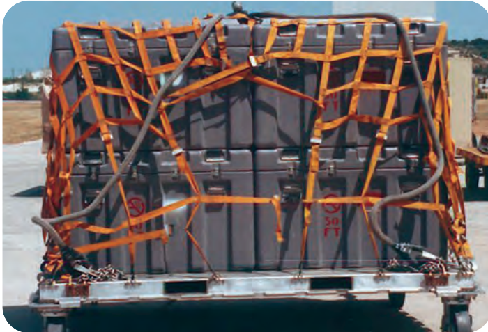
463L INTEX (Internal/External) Multipurpose Aircraft/Helicopter Pallet shown with optional casters and cargo net
