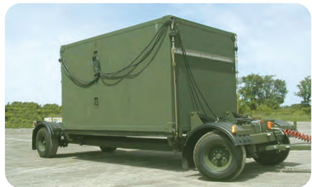
S-280 C/G Shelter shown loaded onto HSMWS
