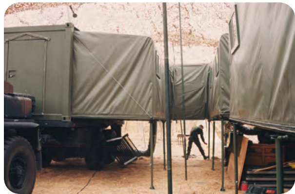
Center vestibule can be used when MECCs are set up on truck level or on ground surface
