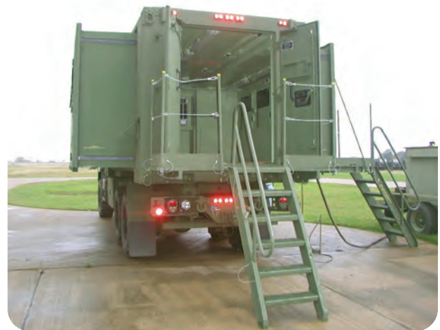
Rear view of M1087 Expandable Van Shelter shown mounted onto a FMTV 5-ton truck (stairway and platform not supplied)
