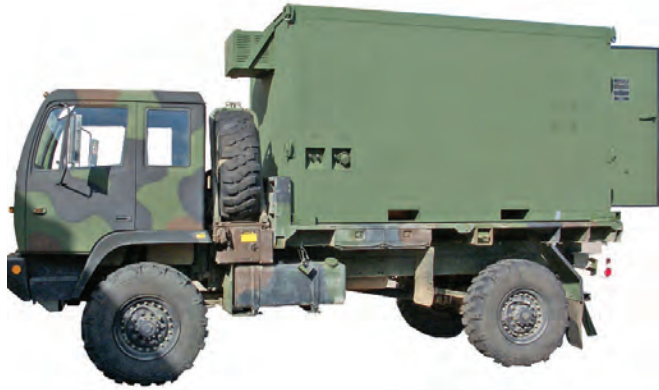
Mobility Shop Container for the LMTV is shown loaded on a standard LMTV truck
