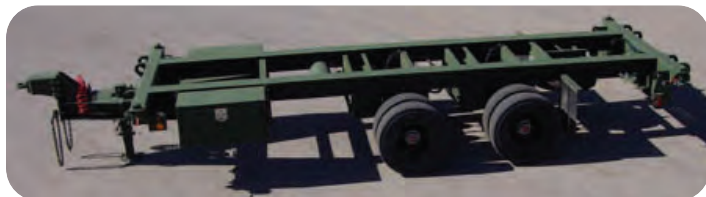
ISO Mobility Trailer is available in 15,000 lb., 18,000 lb., and 28,000 lb. payload capacity
